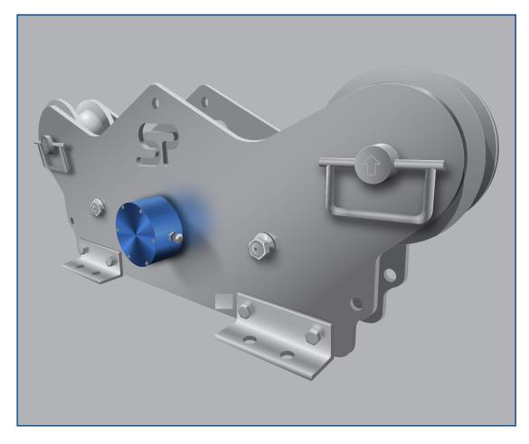
Straightpoint's Running Line Dynamometer TIMH range is built with dockside, marine, offshore, towage and salvage applications in mind. It is particularly useful where there is no anchor or dead end on the line to rig a Straightpoint Radiolink or Loadlink digital dynamometer to measure tension force.
